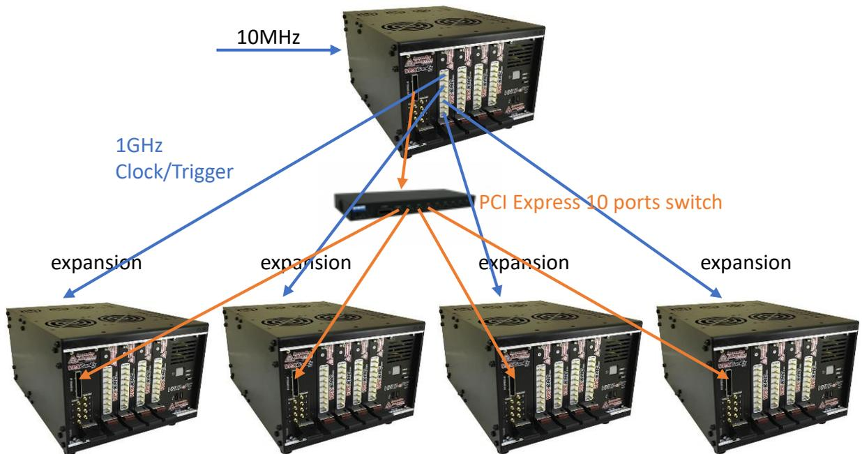
Figure 4. Scalable master-slave system hosts 16 of X6-1000M modules for 16 qubits
