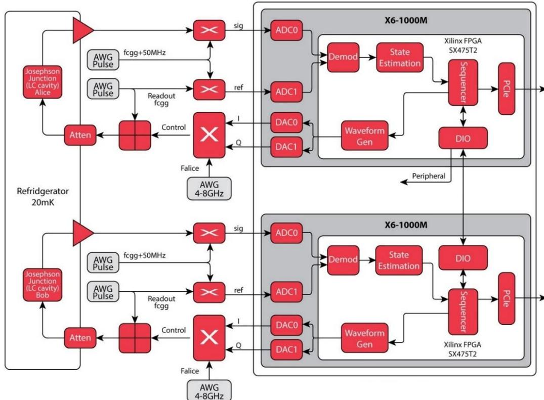
Figure 3. Two entangled qubits using two X6-1000M modules
