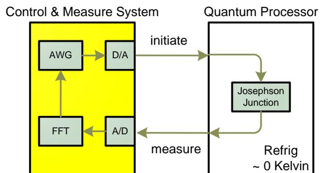
Figure 1. Simplified semiconducting quantum processor physical layer
